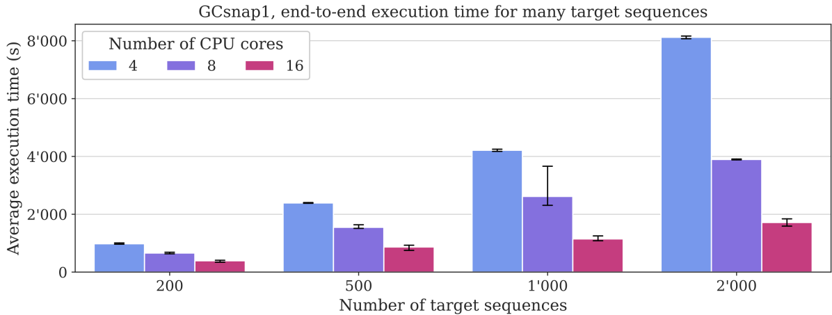
Figure 3.2: Average end-to-end execution time of GCsnap1 over 5 repetitions with different numbers of CPU cores and input targets. Error bars represent the minimum and maximum over the 5 repetitions. Experiments were conducted on an AMD EPYC 7742 CPU with 64 CPU cores. Not all repetitions finished.
