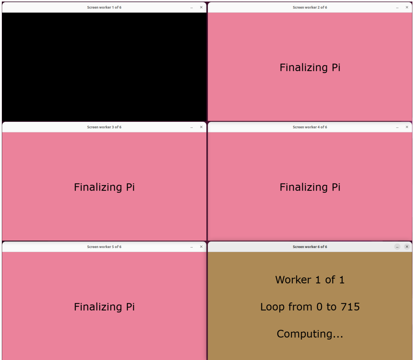
Figure 21: Ranks in the group red combined the individual results and are computing Pi. The single worker from gold is still occupied with iterating. Picture taken while executing the 'How much Pi you like?' application on our own individual machine, allowing up to 6 MPI ranks.
