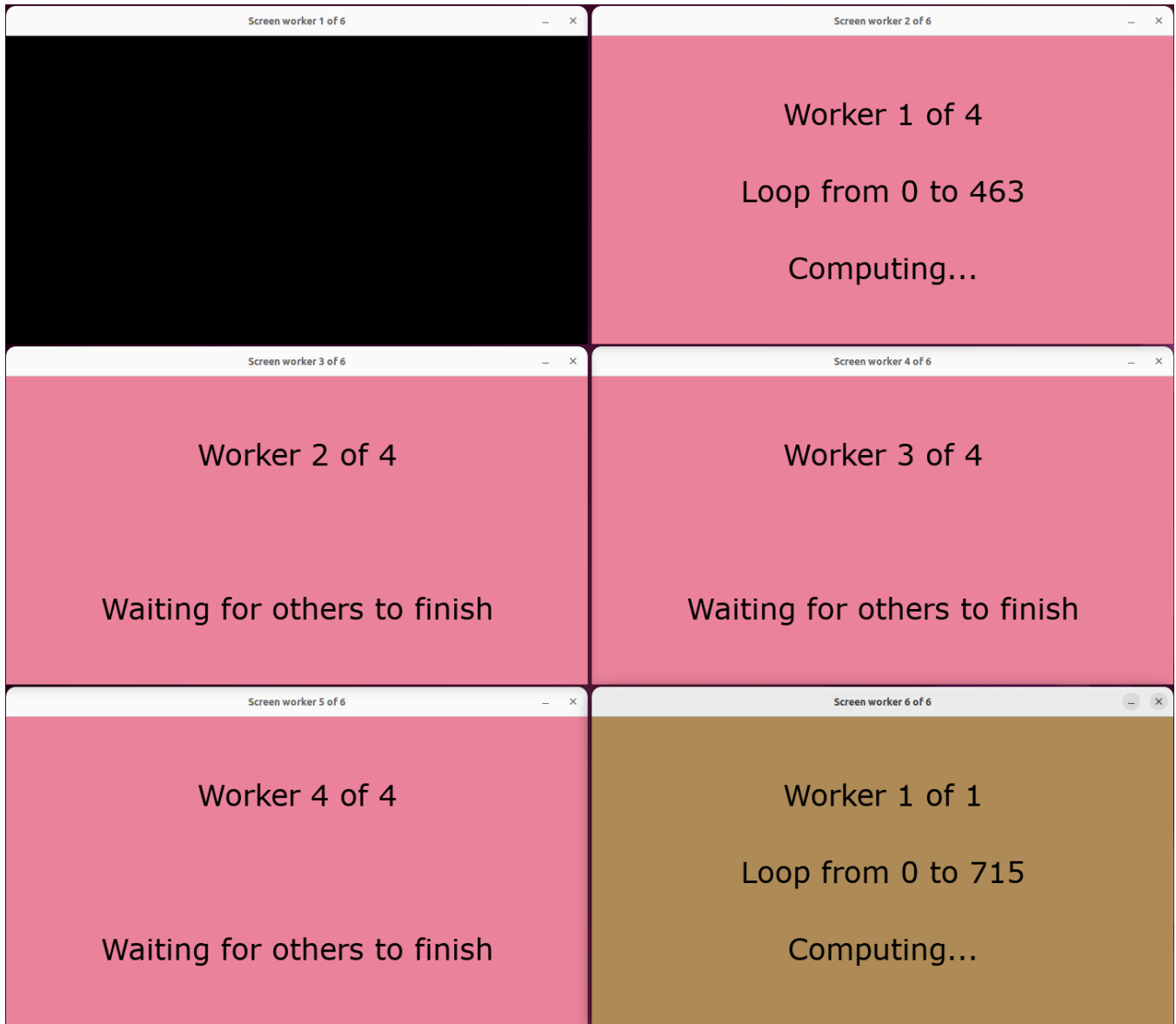
Figure 20: Ranks within a group wait for all to finish, being able to combine the results. 3 ranks in the red group have already completed their workload. Picture taken while executing the 'How much Pi you like?' application on our own individual machine, allowing up to 6 MPI ranks.
